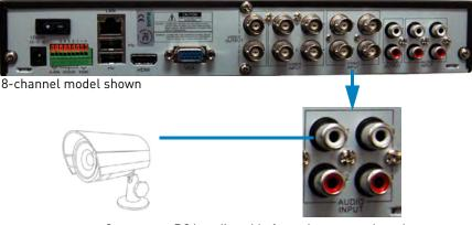
Connect an RCA audio cable from the camera into the corresponding Audio INPUT port
